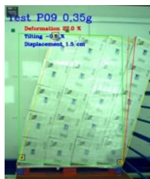
Dynamic deformation P9 to 0.35 g
