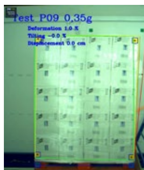
Initial deformation P9 at 0.35 g
